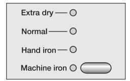
Press the Drying level button repeatedly until the indicator light for the drying level you want lights up.
